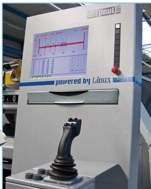
Fig. 4 NCD ripping pattern control
