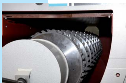
Fig. 4: The saw shaft is located below the insert table
