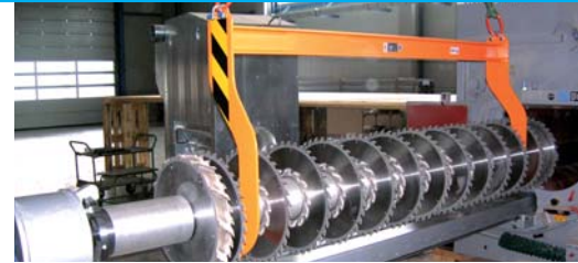
Fig. 5: Special crane hook for transporting the heavy saw shaft
