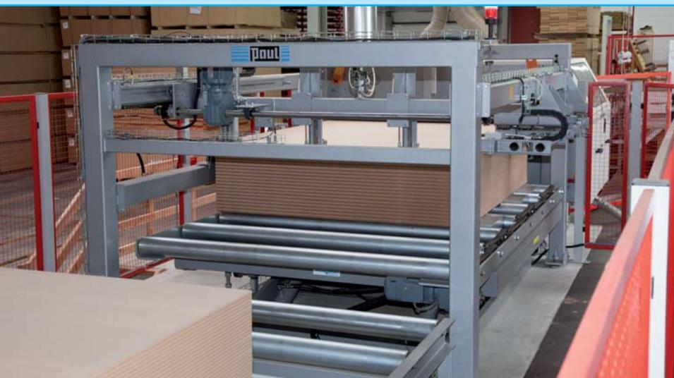
*Fig. 27: Multirip saw with automatic feeding system in the production of strips*
