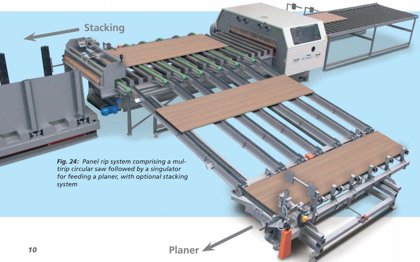
*Fig. 24: Panel rip system comprising a multirip circular saw followed by a singulator for feeding a planer, with optional stacking system*
