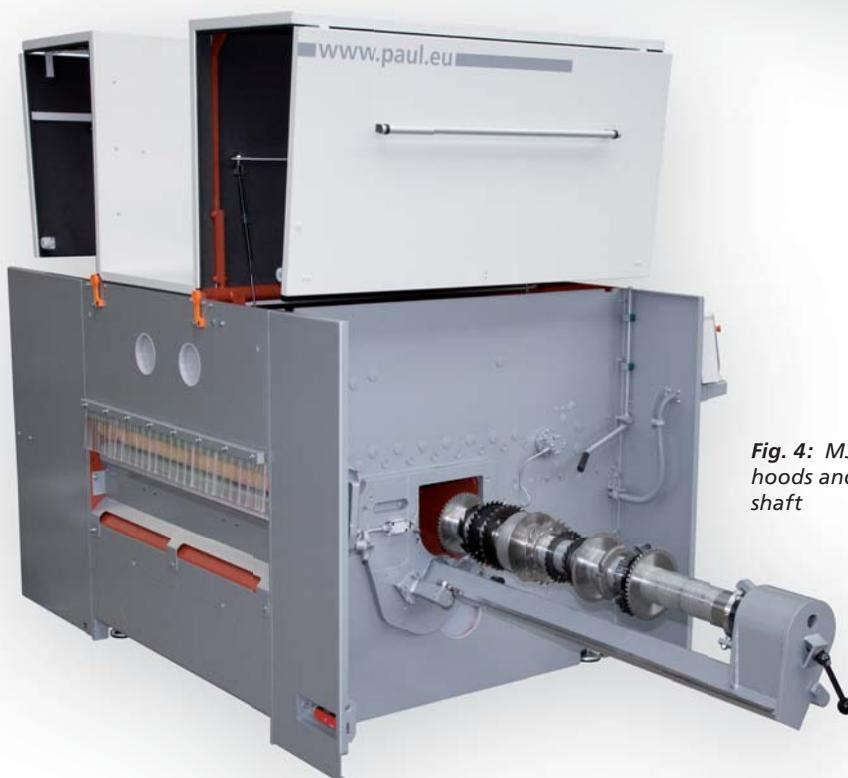
Fig. 4: M34 with opened hoods and extracted saw shaft
