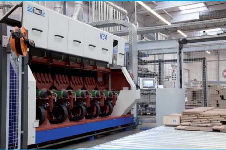
Fig. 7: K34M with 1800 mm opening width ripping particle and MDF panels
