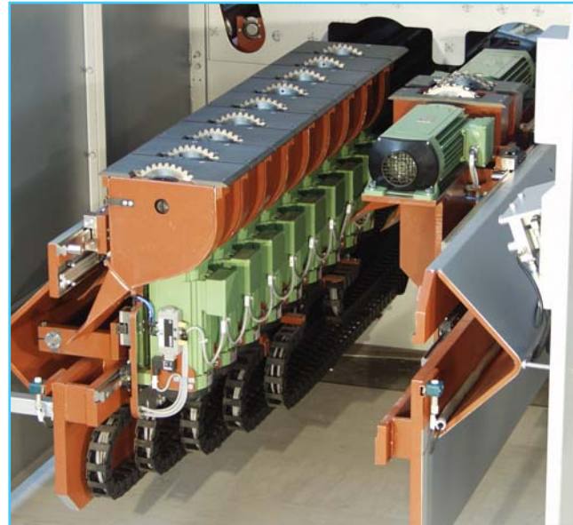
Fig. 6: Saw heads in parking position
