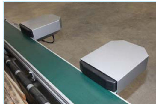
Fig. 12 Fully enclosed ejection stations for high safety
