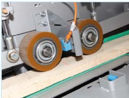
Fig. 9 Separate measuring station for recognition of the crayon mark positions
