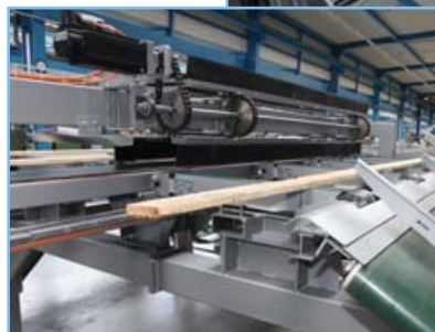
Fig. 17 Distribution to two cross-cut stations
