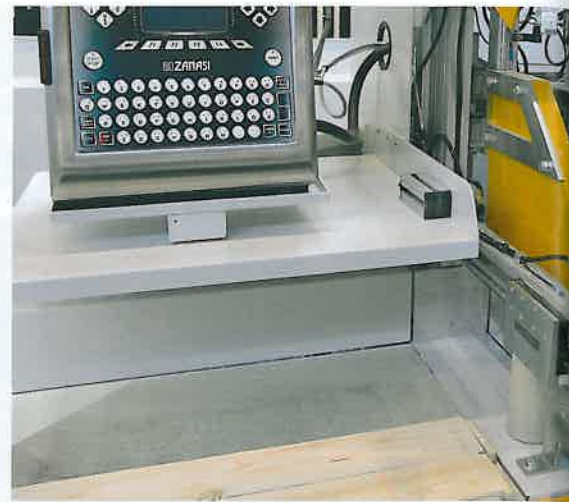
Crosscut saw with printing unit: Salvador exhibited its Superpush 250 with integrated non-contact printing unit (right) which can apply marking, barcodes and lettering (small photo) on wood at normal production speeds
